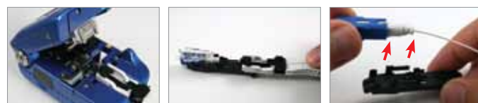
▶ 1 Cutting Fiber ▶ 2 Inserting Fiber ▶ 3 Take Out Connector
